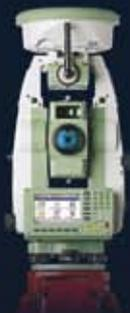
**SmartStation – Total Station with integrated GPS.**
